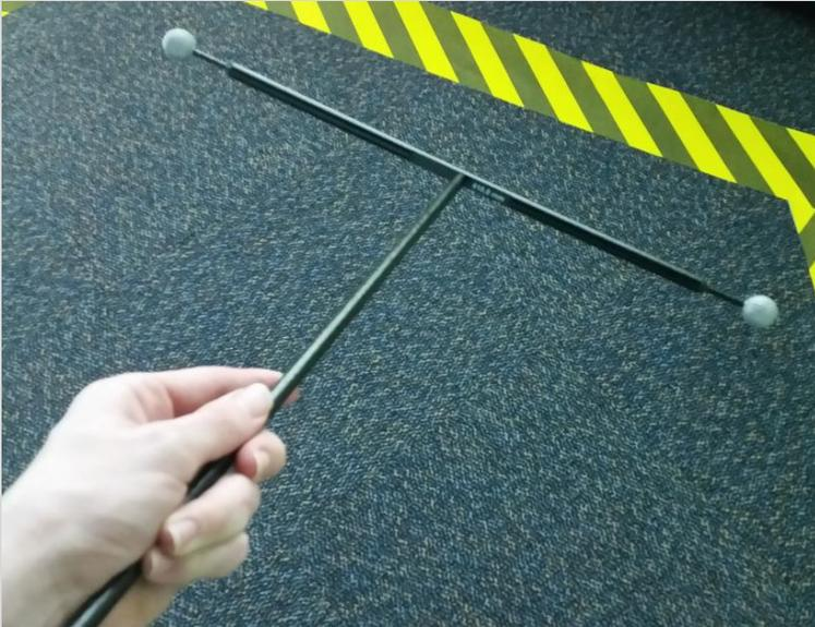
**Room Calibration:** The marker distances is set to 410 and the coordinate system specified is power wall, as this is what getReal and track3d use. A duration of 2 minutes is used for the calibration time to ensure nearly full 100% coverage of the calibration.
